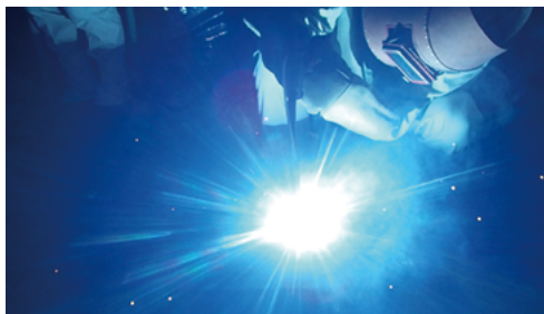
Pulsed gas MAG welding method, a new low-sputter welding method
