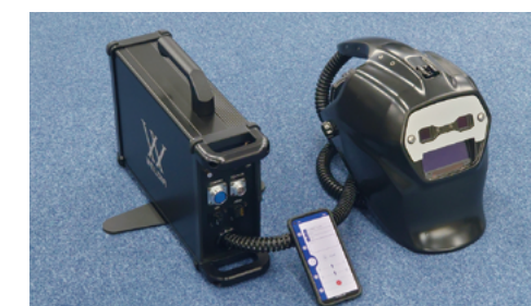
3D Digital Welding Mask System that achieves DX in the transfer of welding skills
