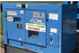
Bio-diesel fuel (B100 fuel) dedicated generator (National Route 7 Yachita District Bridge Superstructure Construction)
