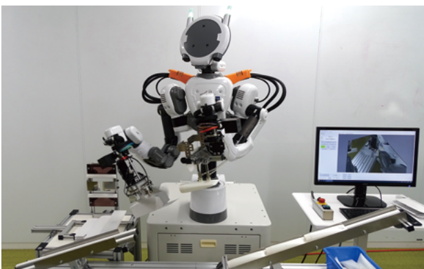
NEXTAGE Fillie humanoid robot and Cobako box packing system
